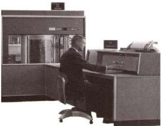
1956: IBM 305 RAMAC computer with hard disk (5MB/1,200RPM)
